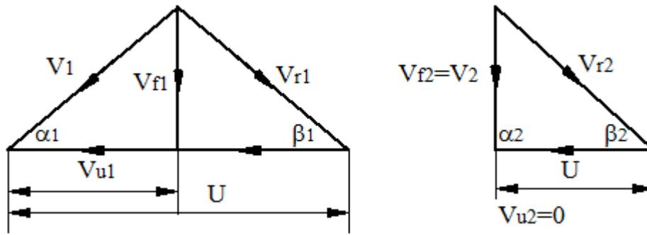
Fig. 4.6 Velocity triangles for Kaplan turbine
