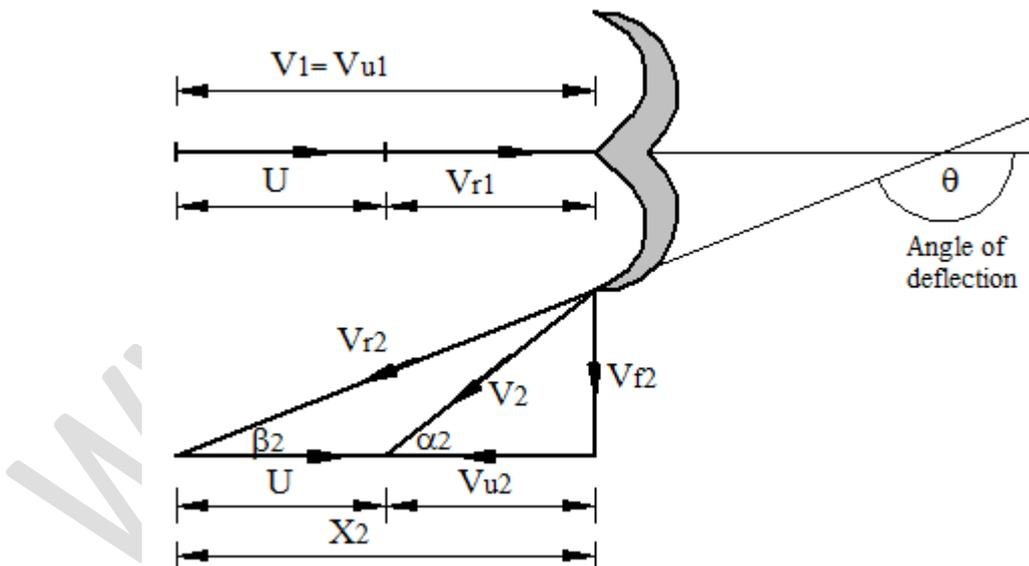
Fig. 4.2 Velocity triangles for Pelton wheel turbine
