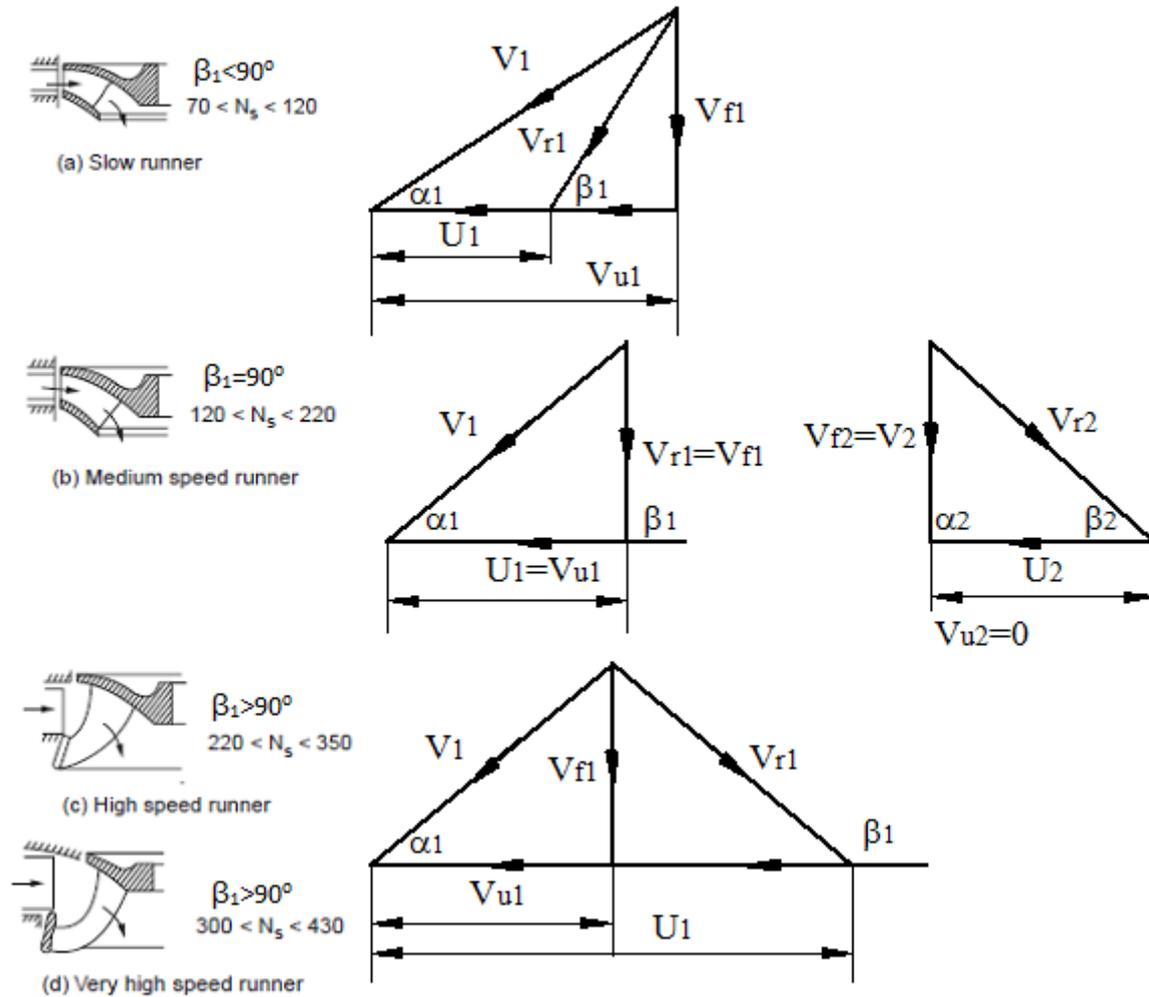
Fig. 4.4 Velocity triangle for Francis turbine
