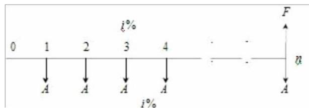
**Fig.1.8** Cash flow diagram of equal-payment series sinking fund.
